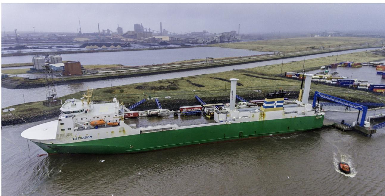
Spinning cylindrical sails can be used on large ships to reduce greenhouse gas emissions and propel them forward. Image credit - Norsepower
