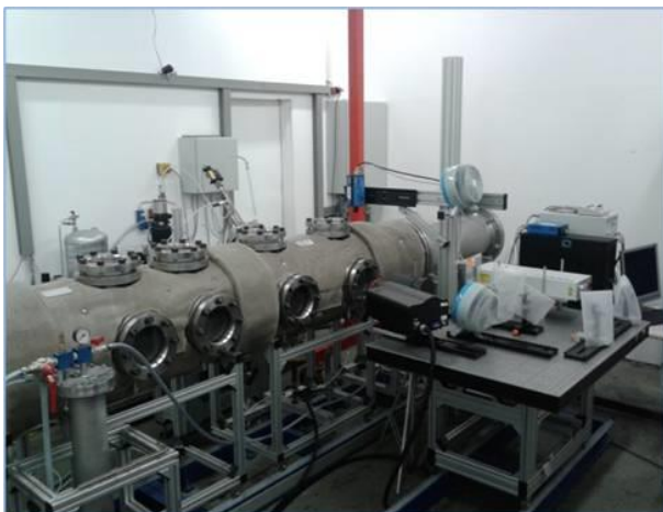
Figure 15: Hot exhaust gas flow test rig for testing area injectors evaporation and mixing
