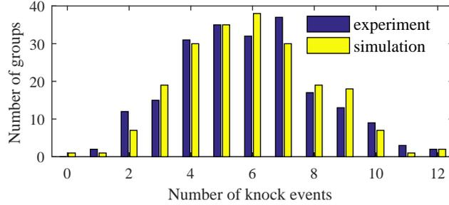
Figure 5. Histogram of knock events: simulation vs. experiment.
