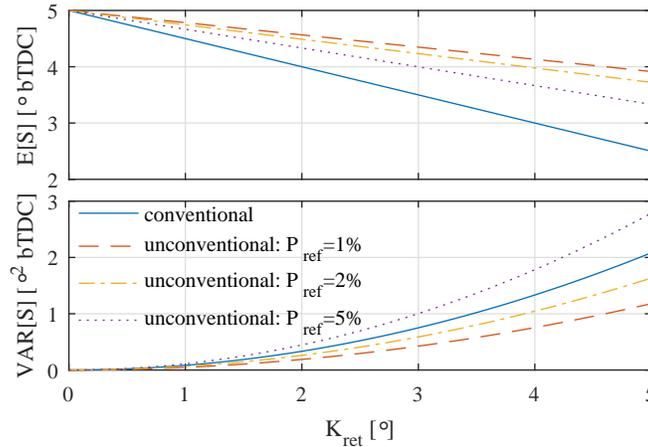
Figure 8. Analytic spark timing average ( $E[S]$ ) and variance ( $VAR[S]$ ) of the conventional and unconventional controllers for different values of  $K_{ret}$  and  $P_{ref}$ .
