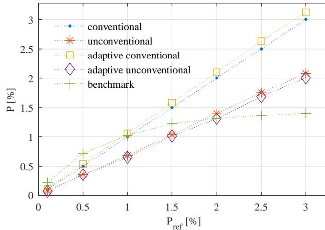
Figure 15. Actual knock rate ( $P$ ) vs. reference probability ( $P_{ref}$ ). The other parameters are equal to the values used for the reference point.
