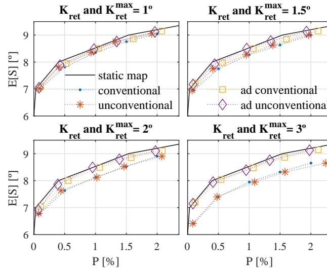
Figure 16. Spark timing average for different values of  $K_{ret}$ ,  $K_{ret}^{max}$  and  $P_{ref}$ . For the adaptive strategies  $K_{ret}^{min} = 0.1$ .
