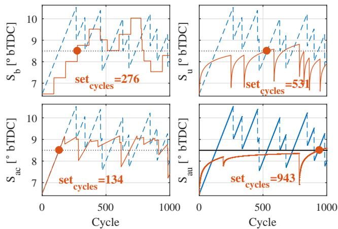
Figure 25. Evolution of the spark timing starting from retarded condition.
