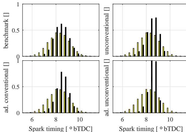
Figure 14. Comparison of the spark timing distribution.
