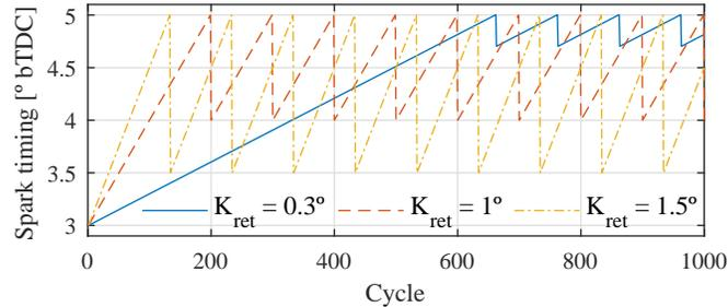
Figure 6. Examples of the evolution of the conventional controller under the assumption of stable operation.  $P_{ref} = 1\%$ ,  $N_{ref} = 100$  cycles.
