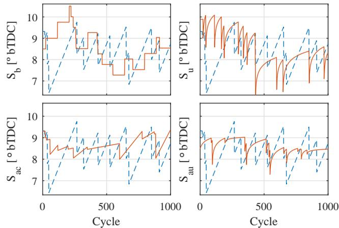
Figure 22. Experimental example at steady-state operation. In each subplot the conventional controller (dashed line) is compared with the benchmark (top left), the unconventional (top right), the adaptive conventional (bottom left), and the adaptive unconventional controllers (bottom right).
