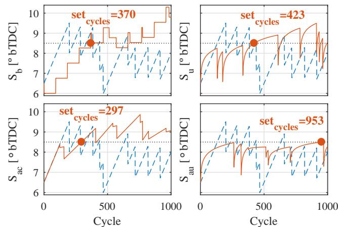
Figure 19. Settling time starting from retarded timing. The conventional controller presents a settling time of 133 cycles.
