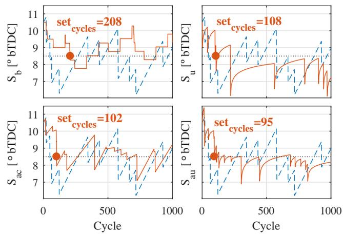
Figure 24. Evolution of the spark timing starting from advanced condition.
