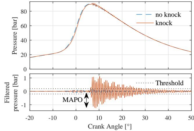
Figure 1. Pressure trace and MAPO index for knocking and non-knocking cycles with the same ignition angle.
