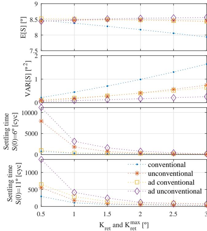
Figure 20. Sensitivity to  $K_{ret}$  and  $K_{ret}^{max}$  (the other parameters are equal to those shown in the steady-state comparison).
