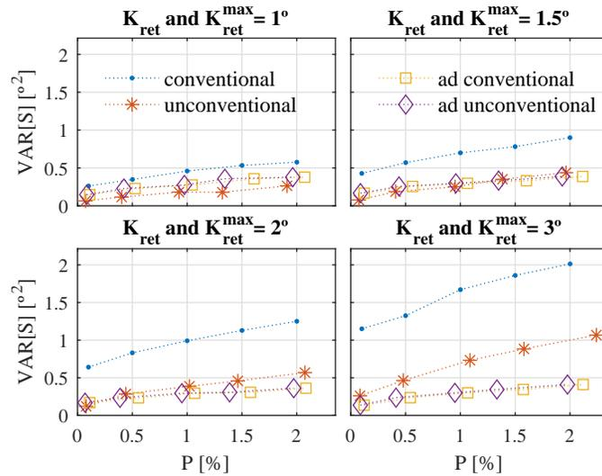
Figure 17. Spark timing variance for different values of  $K_{ret}$ ,  $K_{ret}^{max}$  and  $P_{ref}$ . For the adaptive strategies  $K_{ret}^{min} = 0.1$ .
