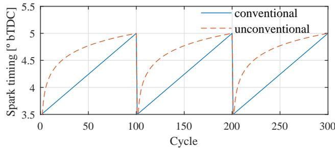
Figure 7. Unconventional vs. conventional controller evolution.  $K_{ret} = 1.5^\circ$ ,  $P_{ref} = 1\%$  and  $N_{ref} = 100$  cycles.
