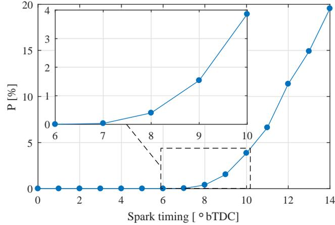
Figure 3. Average knock rate vs. fixed spark timing.
