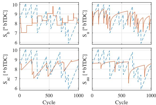
Figure 13. Simulation example at steady-state operation. In each subplot, the conventional controller (dashed line) is compared with the benchmark (top left), the unconventional (top right), the adaptive conventional (bottom left) and the adaptive unconventional controller (bottom right).
