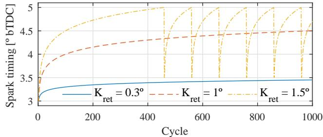
Figure 10. Examples of the unconventional controller evolution under the assumption of stable operation.  $P_{ref} = 1\%$ ,  $N_{ref} = 100$  cycles.
