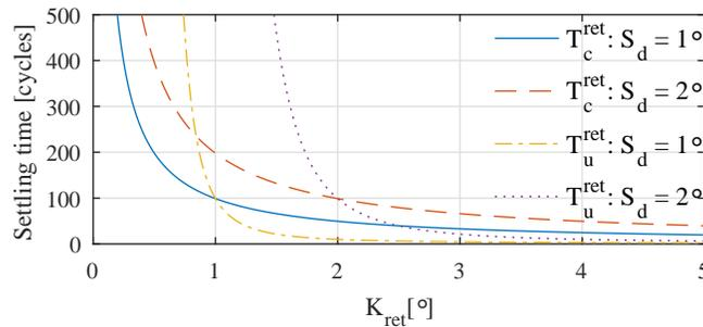
Figure 9. Settling time of the conventional controller ( $T_c$ ) and the unconventional controller ( $T_u$ ) under the assumption of stable operation for different values of  $K_{ret}$  and starting offset ( $S_d$ ).
