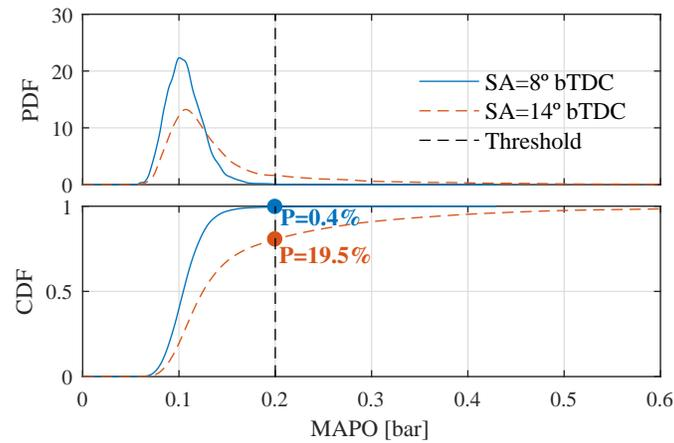
Figure 2. MAPO PDF and CDF for fixed spark angle expressed in  $^{\circ}$  bTDC. The intersection between the MAPO threshold and the CDF defines the average knocking rate at the given spark timing.
