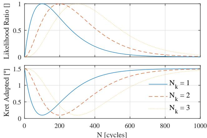
Figure 12. Likelihood ratio and  $K_{ret}$  adapted.  $P_{ref} = 1\%$ ,  $K_{ret}^{min} = 0.1$  and  $K_{ret}^{max} = 1.5$
