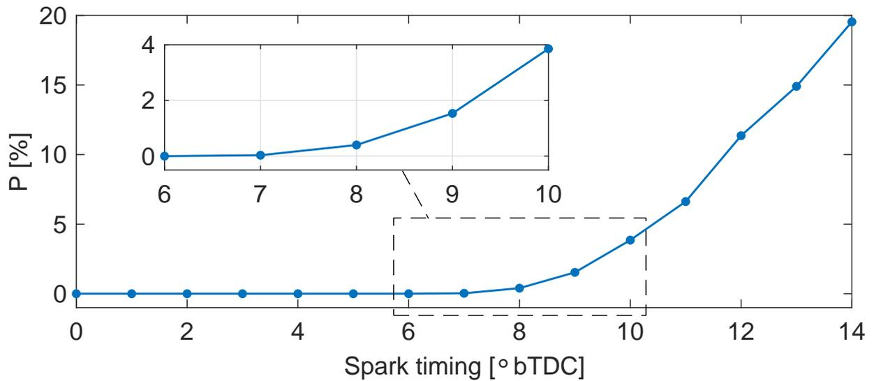
Figure 2. Average knock rate vs. fixed spark timing.
