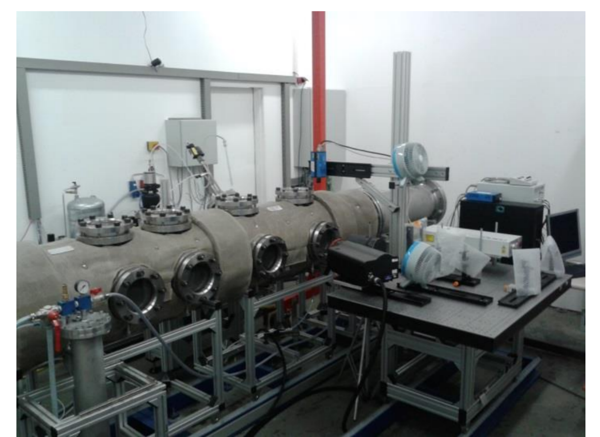
Hot exhaust gas flow rig for investigation of urea injection, evaporation and mixing in Hannover
