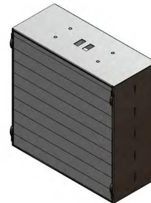
Prototype metallic support for SCR catalyst
