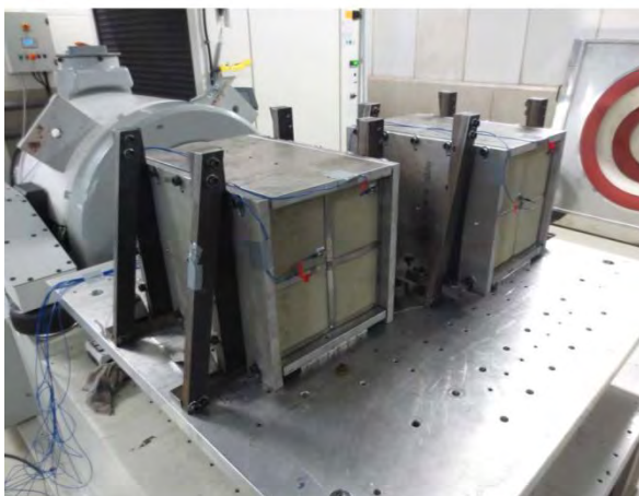
Vibration test setup for extruded SCR catalyst
